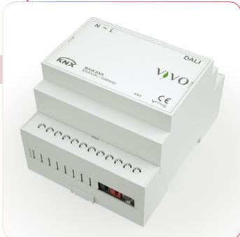
MAIA KNX gateway is a device used for communication between DALI protocol devices and KNX devices. It allows control of up to 64 DALI lights and 16 DALI groups. It is possible to control configured DALI lights or groups through other KNX devices like touch panels, pushbuttons, etc. For each DALI light, this gateway features the most common dimming, switching, brightness value setting, light scenes functions, as well as DALI lights errors feedback.
